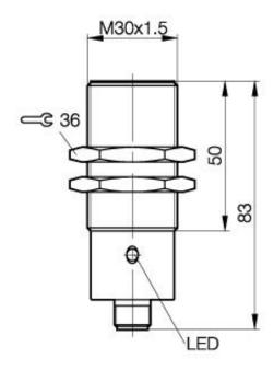
Inductive Sensors BES 516-3028-S 4-C M30x1.5 x 83 normally-closed Sn=10mm shielded
